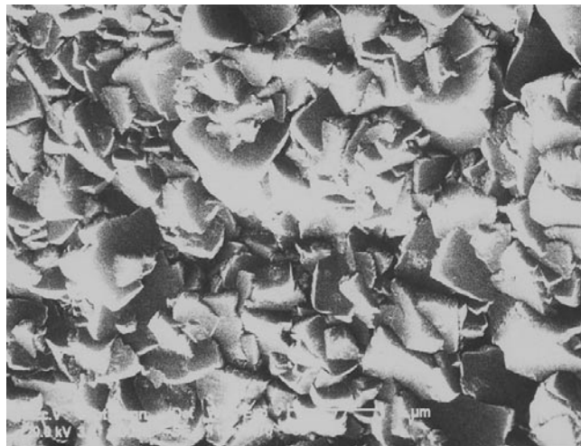
Figure 1. SEM micrograph of diamond film surface grown on PS.
